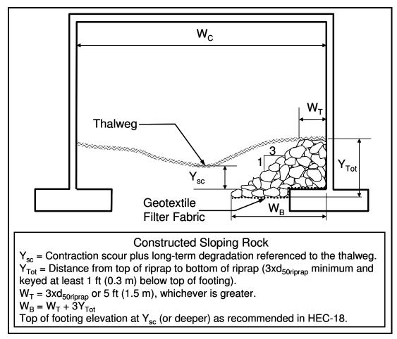
Figure 18.10. Cross Section for Sloping Rock.
