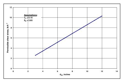
Figure 10.6. Permissible shear stress as a function of the median size of the stone fill.
