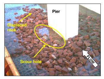
Figure 12.13. Loose riprap after completion of the high velocity comparison test.
