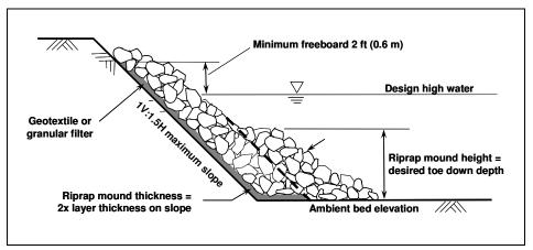
Figure 4.3. Riprap revetment with mounded toe.
