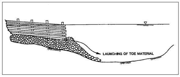
Figure 2.8. Permeable wood-slat fence spur showing launching of stone toe material (after Brown 1985).
