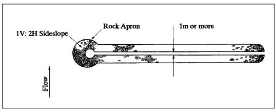
Figure 2.12. Typical straight, round nose spur.
