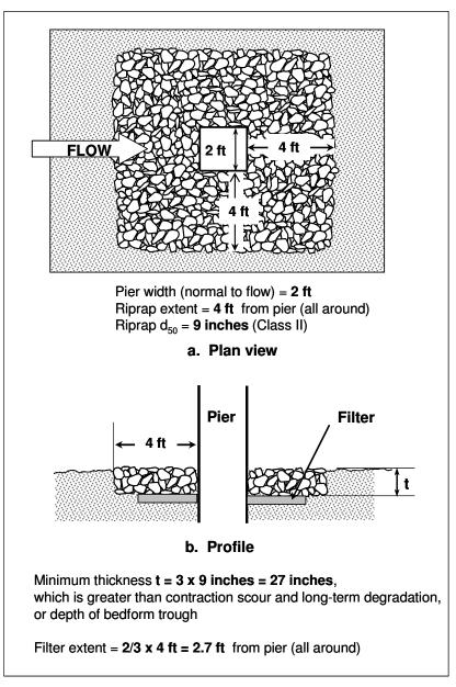
Figure 11.21. Riprap layout diagram for pier scour protection.
