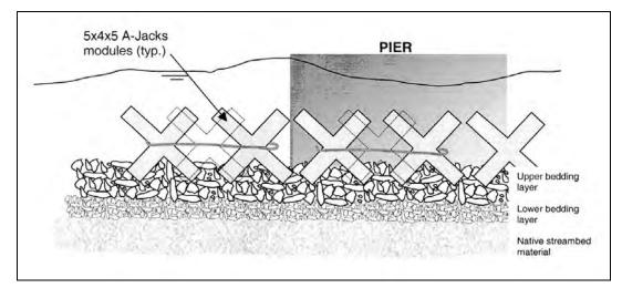
Figure 19.4a. Bedding detail showing two layers of granular bedding stone above native streambed material (Clopper and Byars 1999).
