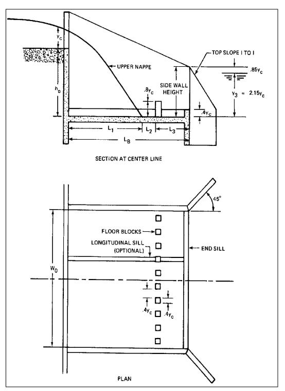
Figure 3.3. Straight drop structure stilling basin.
