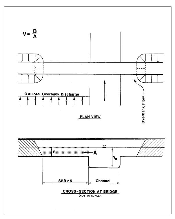
Figure 14.5. Characteristic average velocity for SBR>5.
