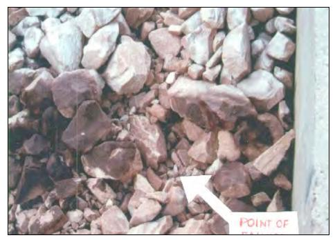
Figure 5.9. Riprap failure in 1997 tests ( $d_{50} = 0.89$  ft (271 mm)).
