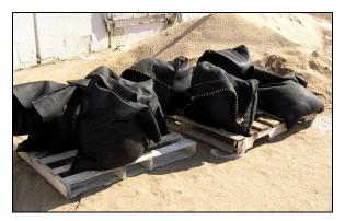
Figure 11.10. Geotextile containers before installation around the pier.
