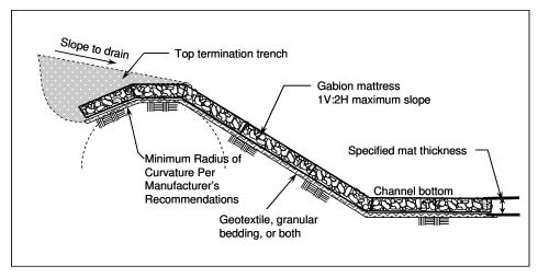
Figure 10.4. Recommended layout detail for bank and bed armor.
