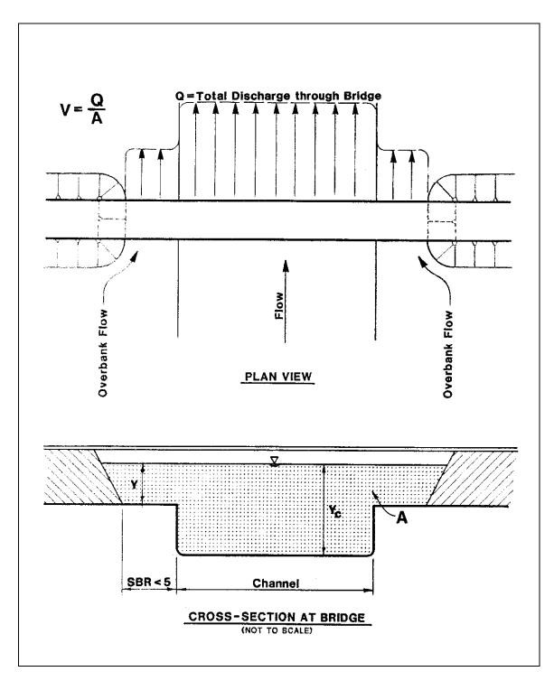
Figure 14.4. Characteristic average velocity for SBR<5.
