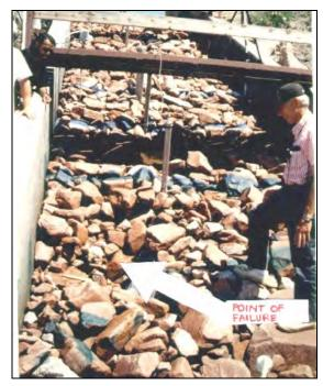
Figure 5.7. Riprap failure in 1994 tests ( $d_{50} = 1.27$  ft (386 mm))
