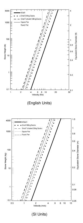
Figure 11.2. Effect of turbulence intensity on rock size using the Isbash approach.
