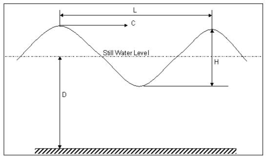
Figure 17.3. Wave characteristics.
