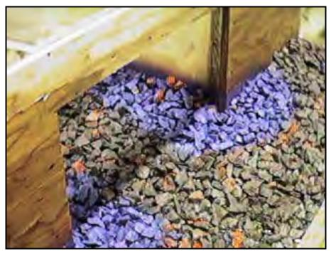
Figure 18.6. Riprap scour protection with a rectangular model (Kerenyi et al. 2003).
