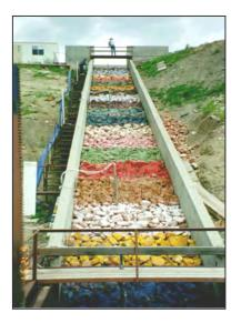
Figure 5.4. Test set up for 1997,  $d_{50} = 0.89$  ft (271 mm).
