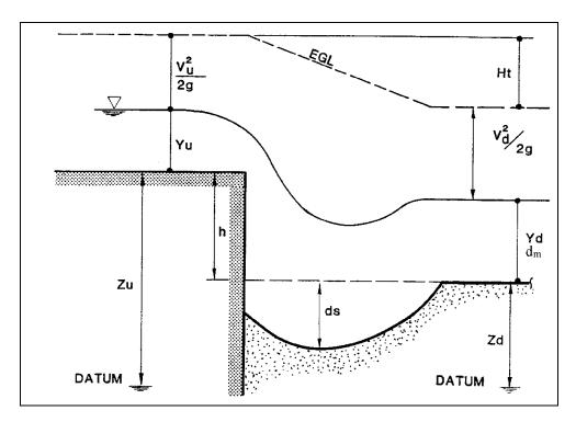
Figure 3.1. Schematic of a vertical drop caused by a check dam.
