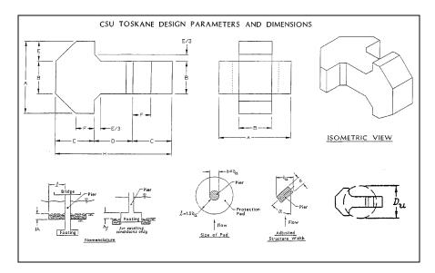
Figure 19.2. Toskane design parameters and dimensions.
