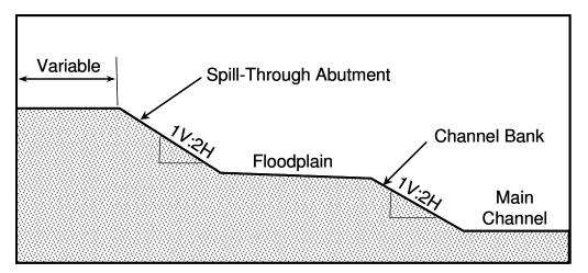
Figure 14.2. Section view of a typical setup of spill-through abutment on a floodplain with adjacent main channel.
