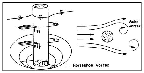
Figure 11.1. Schematic representation of scour at a cylindrical pier.
