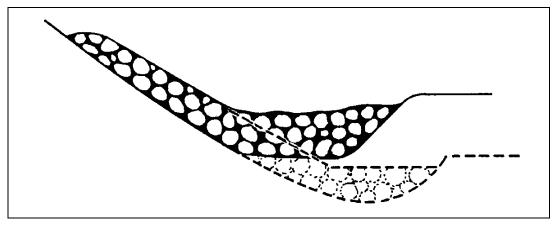
Figure 4.12. Rock-filled trench (after Richardson et al. 2001).
