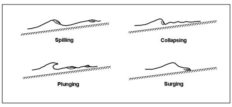
Figure 17.5. Schematic illustration of wave types (from HEC-25).
