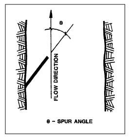
Figure 2.2. Definition sketch for spur angle (after Karaki 1959).
