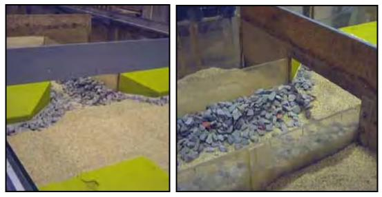
Figure 18.8. MDSHA standard plan after test (Kerenyi et al. 2007).
