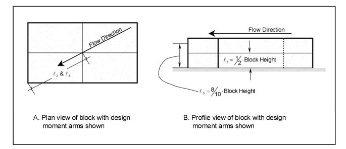
Figure 8.4. Schematic diagram of a block showing moment arms  $\ell_1$ ,  $\ell_2$ ,  $\ell_3$ , and  $\ell_4$ .
