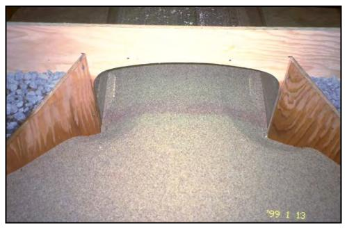
Figure 18.5. Arched model with wing walls (Kerenyi et al. 2003).
