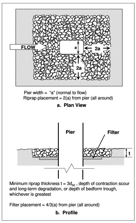
Figure 11.15. Riprap layout diagram for pier scour protection.
