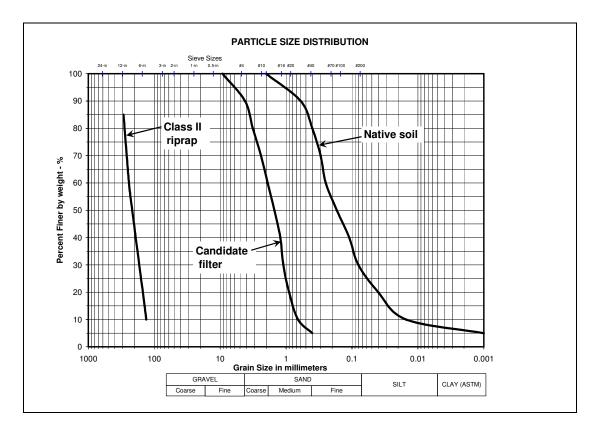
Figure 16.4. Grain size curves for design example.
