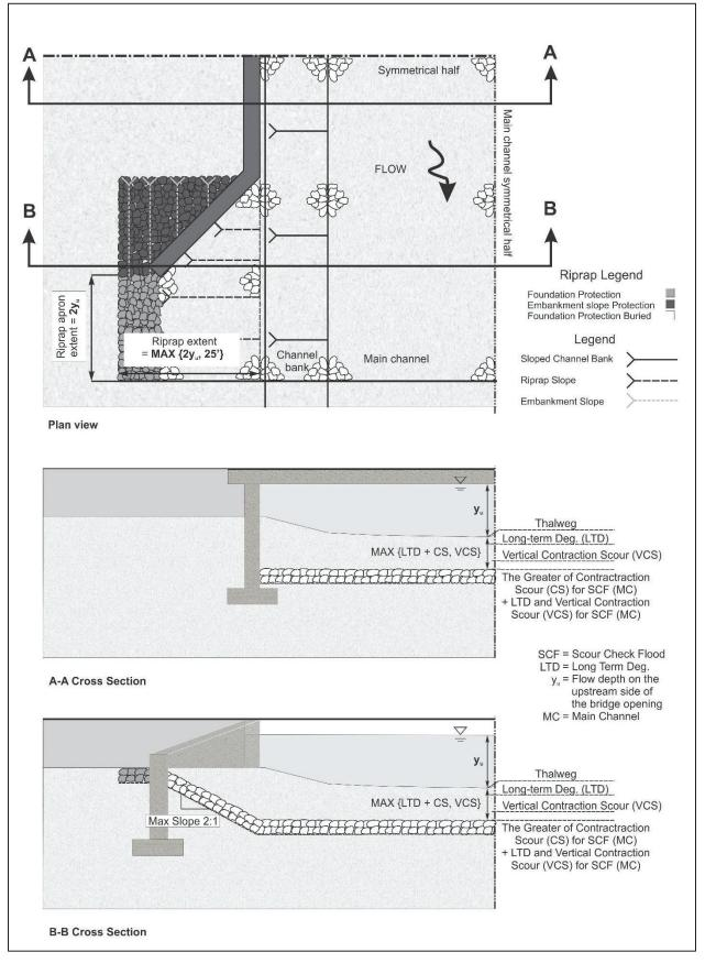
Figure 10: Pressure Flow Scour Countermeasure.
