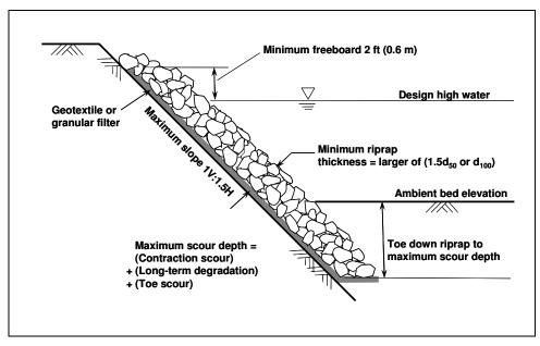
Figure 4.2. Riprap revetment with buried toe.
