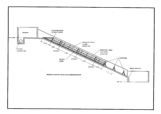
Figure 5.5. Riprap configuration in 1994 and 1995.
