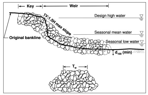
Figure 1.2. Bendway weir typical cross section.
