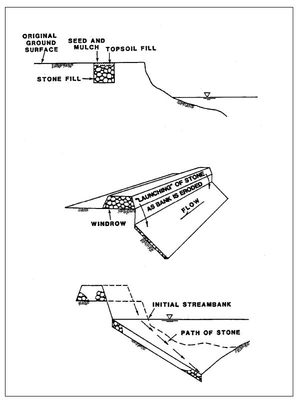
Figure 4.13. Windrow revetment, definition sketch (after USACE 1981).
