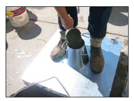
a. Slump cone and test table
