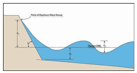
Figure 17.6. Wave runup schematic for freeboard calculations (from HEC-25).
