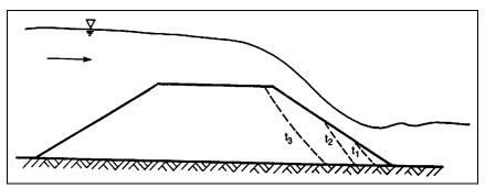
Figure 5.2. Typical embankment erosion pattern with free flow.
