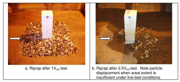
Figure 11.4. Riprap tests under clear-water and live-bed conditions.
