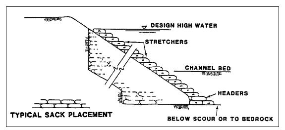
Figure 4.14. Typical sand-cement bag revetment.
