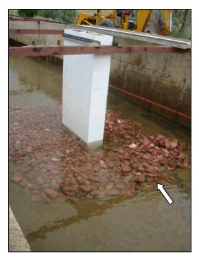
Figure 11.14. Riprap armor over geotextile containers.
