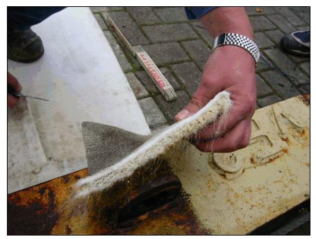
Figure 11.17. Close-up photo of SandMat<sup>™</sup> geocomposite blanket. (photo from NCHRP Project 24-07(2), courtesy Colcrete – Von Essen Inc.)
