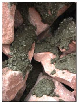
Figure 12.10. Interior of the dry riprap pile (some surface rocks removed).
