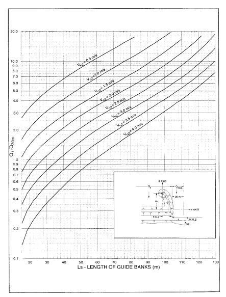
Figure 15.3. SI version of nomograph to determine guide bank length (after Bradley 1978).
