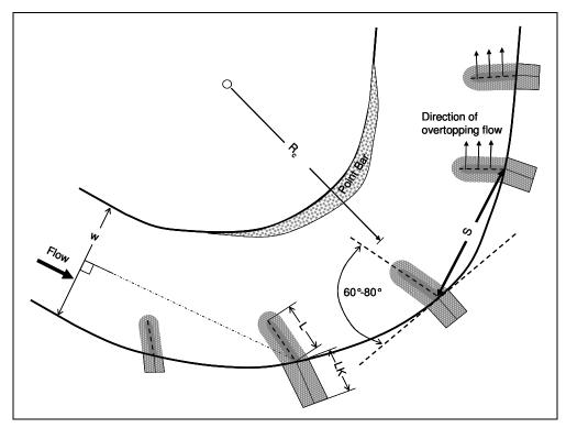
Figure 1.1. Bendway weir typical plan view.
