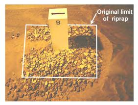
Figure 11.6. Mounded riprap after 2V<sub>crit</sub> test.
