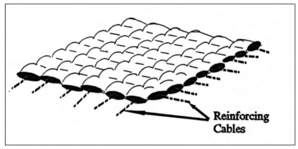
Figure 9.1. Grout-filled mat with reinforcing cables (Fotherby 1995).
