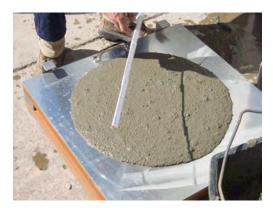
b. Measuring grout slump diameter
