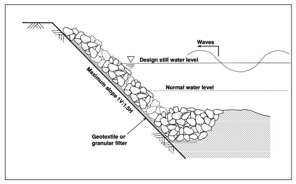
Figure 17.2. Riprap shore protection - typical design configuration.
