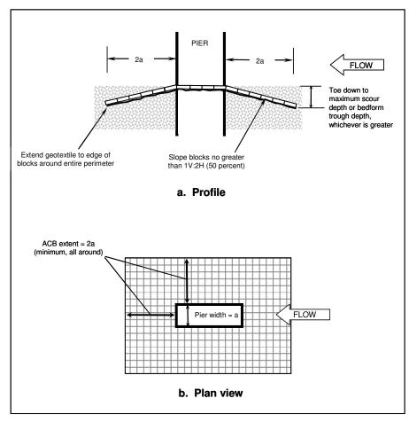
Figure 8.10. ACB layout diagram for pier scour countermeasures.
