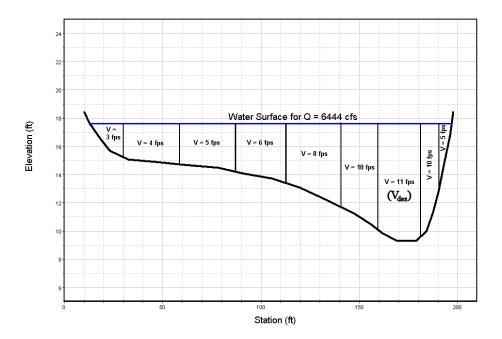
Figure 8.9. Velocity distribution at River Mile 23.4 from HEC-RAS model.
