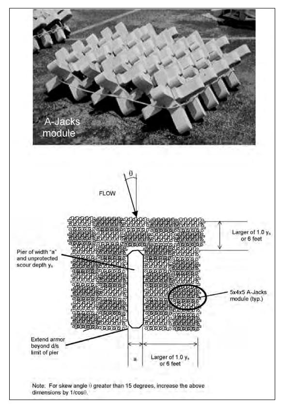
Figure 19.3. A-Jacks modules for pier scour protection.
