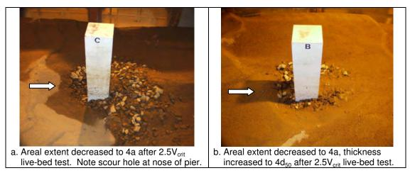
Figure 11.5. Decreased areal coverage riprap tests.
