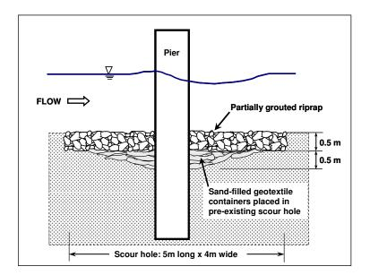
Figure 11.9. Schematic of geotextile container tests.
