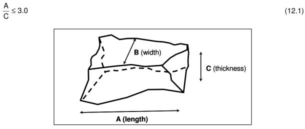
Figure 12.2. Riprap shape described by three axes.
