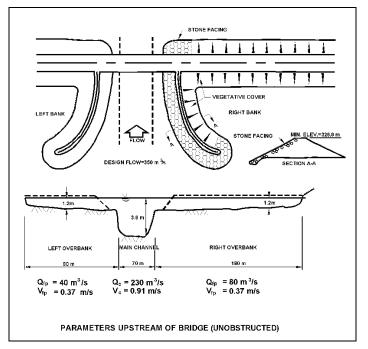
Figure 15.5. Example guide bank design (SI).
