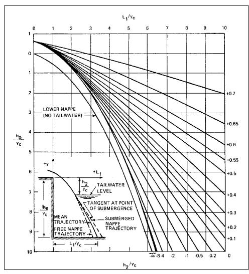
Figure 3.4. Design chart for determination of L<sub>1</sub>.
