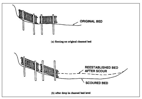
Figure 2.9. Henson spurs (a) resting on original channel bed, and (b) after drop in channel bed level (after Brown 1985).
