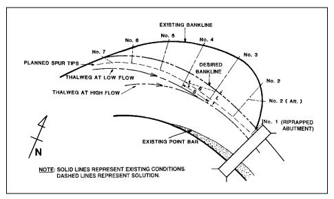
Figure 2.14. Example of spur design.
