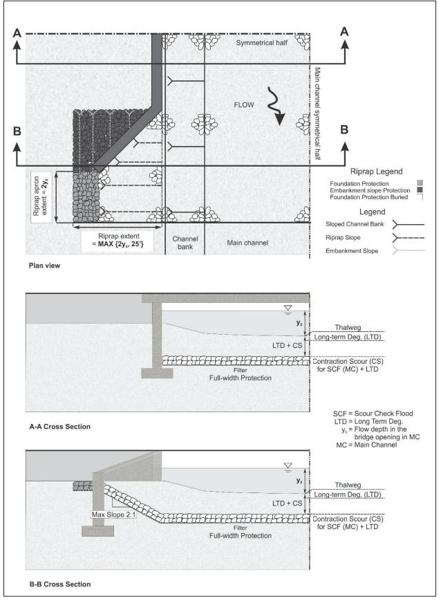
Figure 9: Free-Surface Flow, Narrow-Opening Scour Countermeasure.
