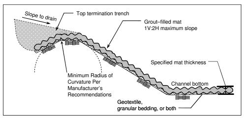
Figure 9.5. Recommended layout detail for bank and bed armor.
