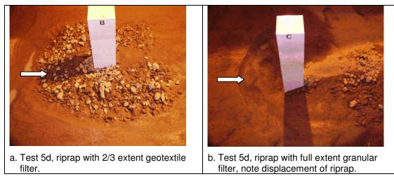
Figure 11.7. Testing of granular and geotextile filters.
