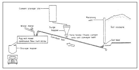
Figure 7.6. Schematic of continuous flow mixing plant for soil cement.<sup>(7)</sup>
