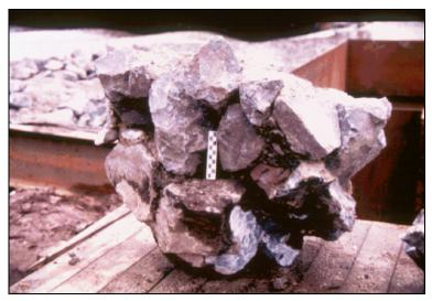
Figure 12.19. Conglomerate produced by spot grouting.
