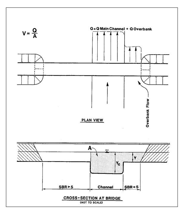
Figure 14.6. Characteristic average velocity for SBR>5 and SBR<5.
