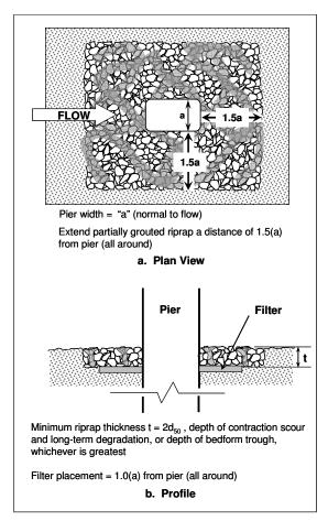
Figure 12.4. Partially-grouted riprap layout diagram for pier scour countermeasures.
