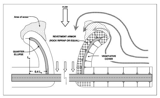
Figure 15.1. Typical guide bank (modified from Bradley 1978).
